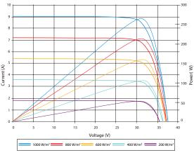
Excellent performance under weak light conditions: at an irradiation intensity of 200 W/m² (AM 1.5, 25 °C), **96.5%** or higher of the STC efficiency (1000 W/m²) is achieved
