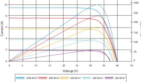
Excellent performance under weak light conditions: at an irradiation intensity of 200 W/m<sup>2</sup> (AM 1.5, 25 °C), **96.5%** efficiency (200 W/m<sup>2</sup>) is achieved
