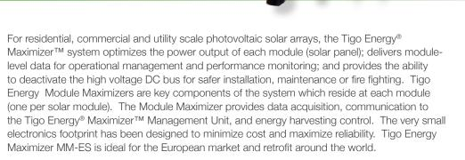
The Tigo Energy output optimization starts with dynamic module balancing – a Module Maximizer (patented) attached to each module manages the energy harvest and sends information to the Maximizer Management Unit for reporting and control. The Tigo Energy Serial Module Maximizer (MM-ES) connects in a series topology. MM-ES maintains best-in-class system conversion efficiencies.
